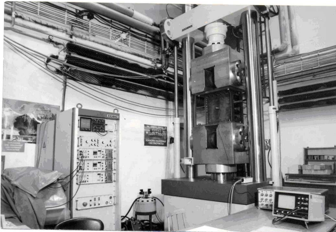
Fig.16: General view of experimental arrangement for the test of thin-walled panel
