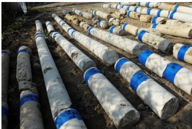
Fig.5: Core samples taken from jet grouting columns (own photo)
