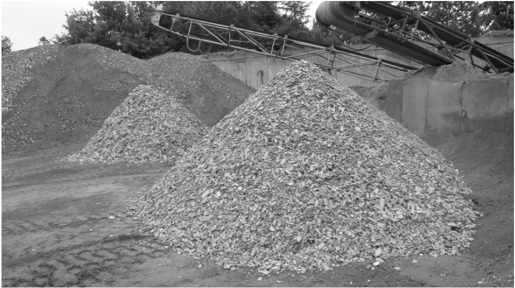
Fig. 1: Ground ceramic waste used as a coarse aggregate
