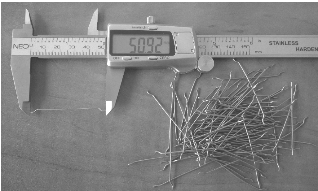
Fig. 2: A geometrical characteristic of used steel fibre
