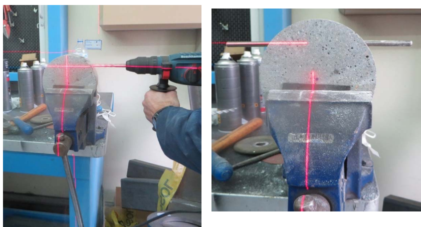
Fig. 3: Threading the steel bars into the holes drilled in the MCT specimen
