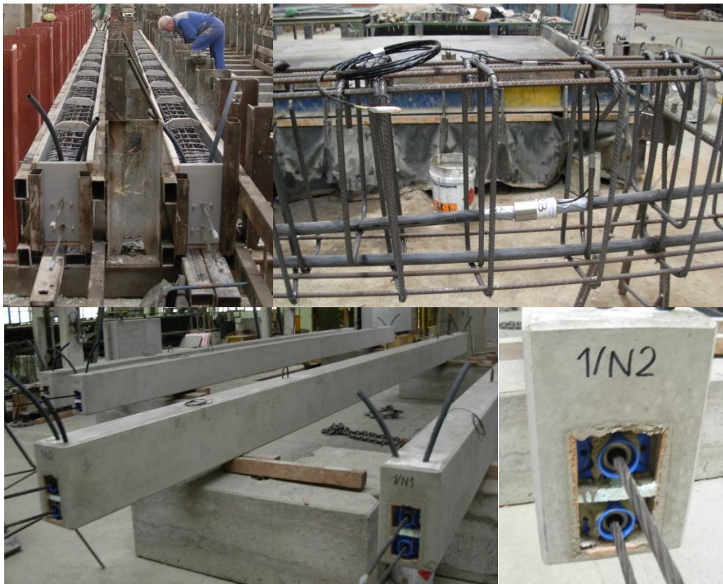
Fig. 3: Preparation and realization of the experimental beams
