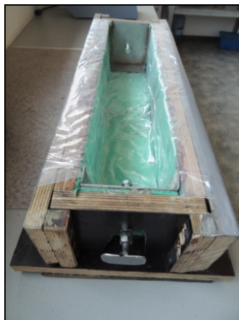
Fig. 4: Mould for measuring the early shrinkage (left), mould in the climatic chamber (right)
