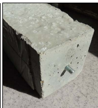
Fig. 5: Reflector of the laser beam and its anchoring
