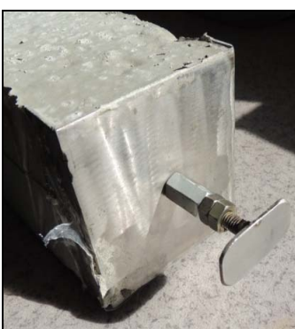
Fig. 5: Reflector of the laser beam and its anchoring
