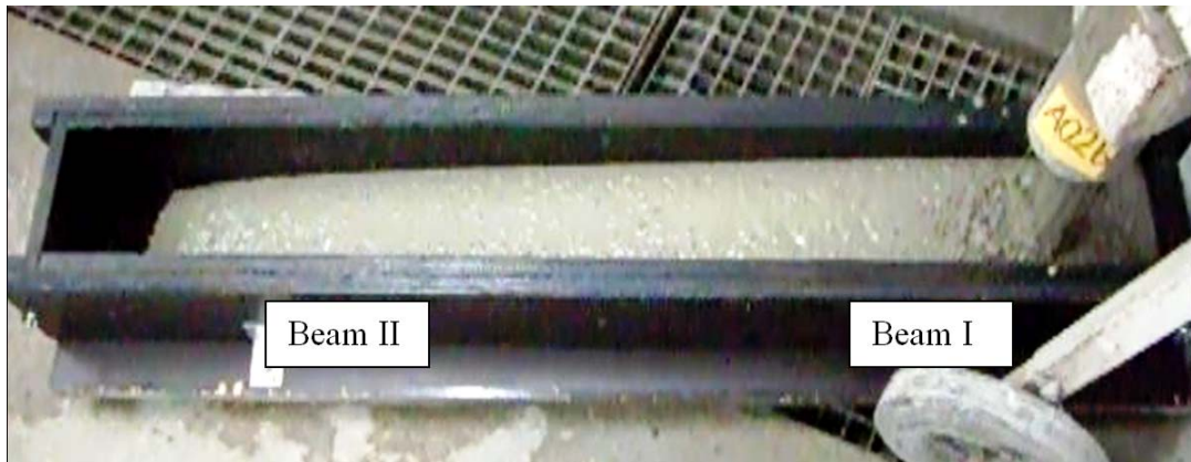
Fig. 1: Forming concrete beams 120×15×15 cm 3 , subjected to further testing as two separate beams
