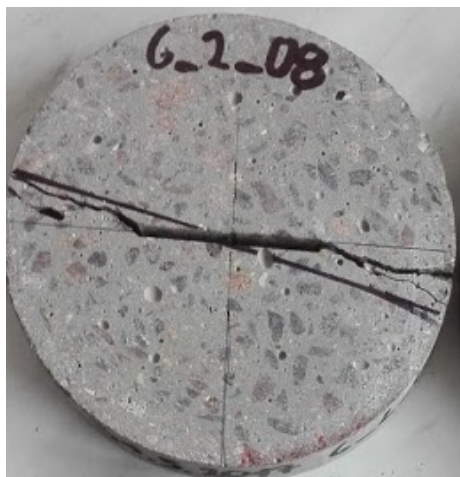
Fig. 7: Actual experimental BDCN test pattern for \alpha = 15^\circ , see [23].
