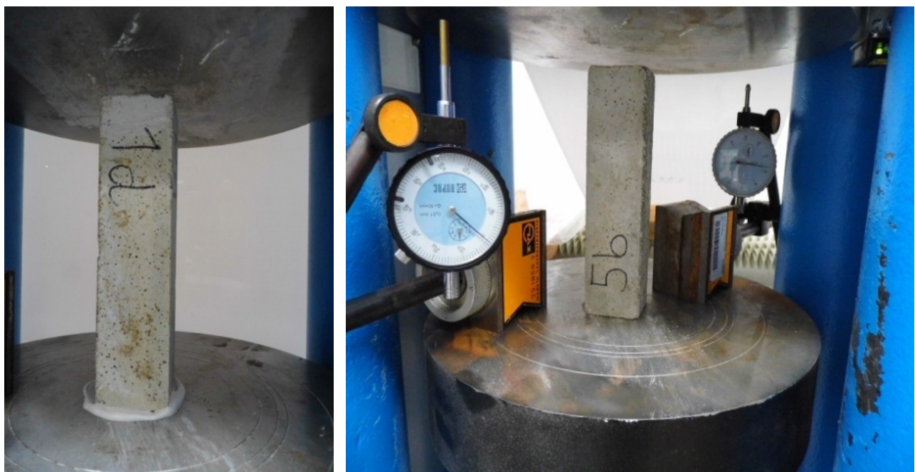
Fig. 2: Destruction tests and measurement of elastic modulus.
