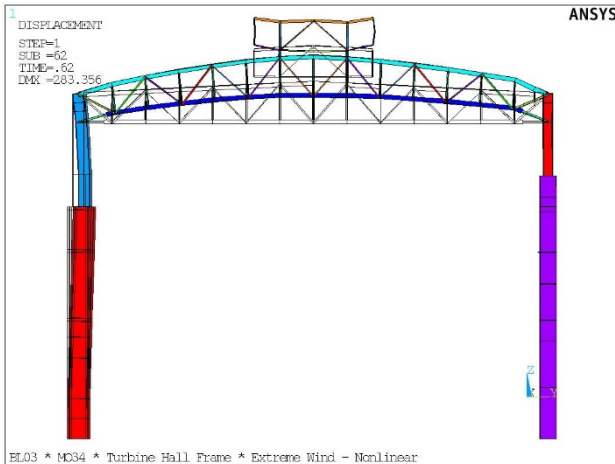
Fig. 8: Deformation of the frame for the HCLPF =4.576 kPa.
