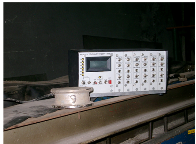
Fig. 2: Sensor with tensiometers (own source).
