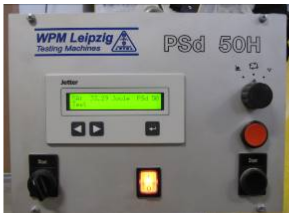
Fig. 1, 2: The Charpy hammer PSd 50H
