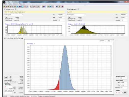
Fig. 5: Histogram - reliability function G_{fail} in 54 years – propagation from the edge
