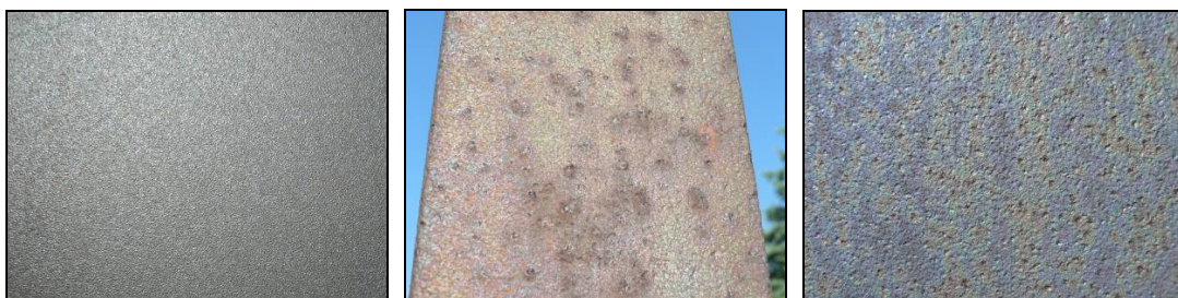
Fig. 1: Appearance of the patina on the directly wetted surfaces (left – patina on the column of a load-carrying structure of a TV mast transmitted in Hošťálkovice, middle – patina on the angle bar of the power grid mast in Ostravice, right – patina on a mast in a crane track in Ostrava-Vítkovice)
