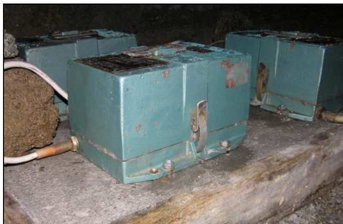
Fig. 2: Seismometers SM3 are anchored to a concrete pillar.
