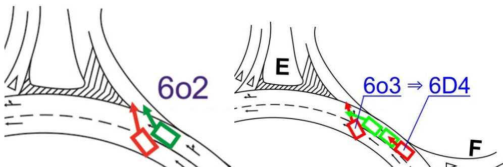
Figure 7: Possible conflict situations during exiting double-line circulating roadway to single-line exit
