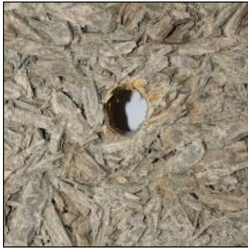
Fig. 8: Hole deformation after destructive testing for dowel with diameter 12 mm
