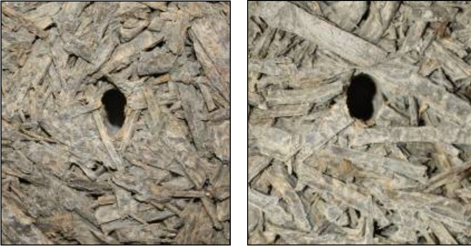
Fig. 6, 7: Hole deformation after destructive testing for dowel with diameter 6 and 8 mm
