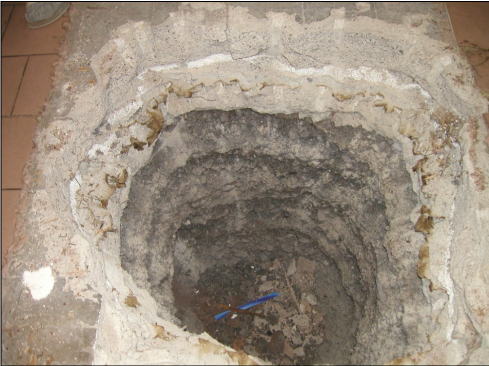
Figure 7: Sampling probe dug inside of the building
