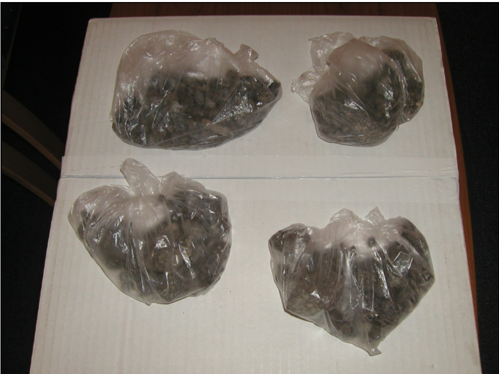
Figure 8: The analyzed slag samples taken from the probe dug in sub-soil of the building
