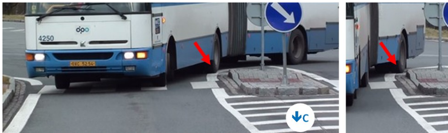
Fig. 8: The bus driving over visual island (conflict situation 2j so 1-O1K), or near the curb of refuge island (conflict situation 2j o 1-O1K); the left picture shows driving over guide lane by left wheel of the second axle, the right picture shows the third axle the same bus
