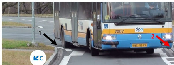
Fig. 9: The bus driving near the curb of refuge island (No. 1; conflict situation 2j o 1-O1K); 2 ... driving by left profile of the bus over guide strip
