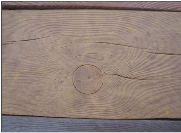
Fig. 5: Prototype of geopolymer wood imitation [15]
