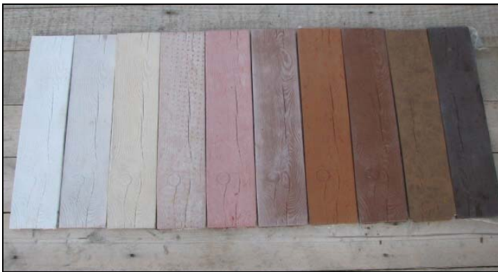
Fig. 6: Prototypes of geopolymer wood imitation - color scale [15]
