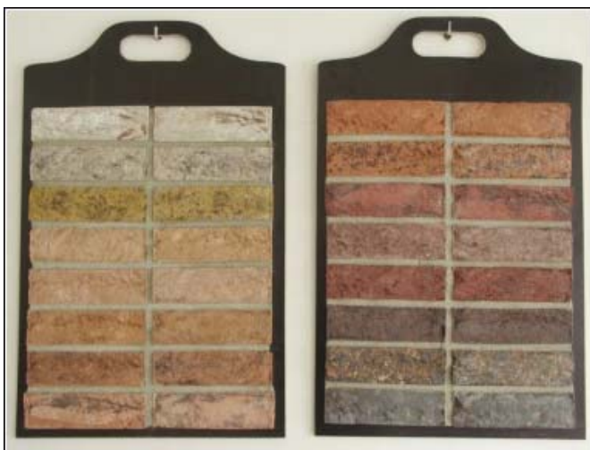
Fig. 4: Prototype of geopolymer brick imitation [15]
