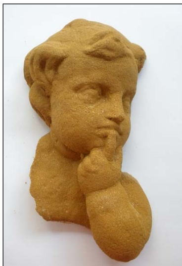
Fig. 1: Detail of stone sculptures copy, that was created by stomping of geopolymer mixture based on blast furnace slag, metakaolin and waste sand from kaolin washing [24]
