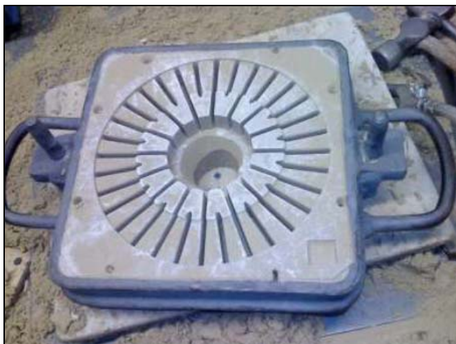
Fig. 3: Part of molds for bronze casting [30]
