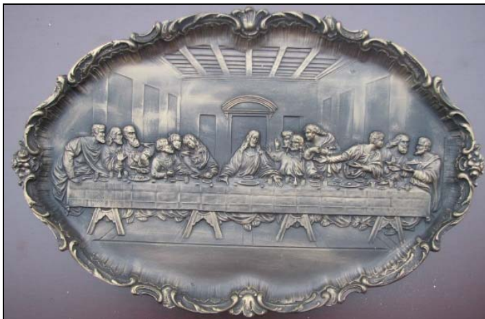
Fig. 7: Prototype of geopolymer brass imitation [15]
