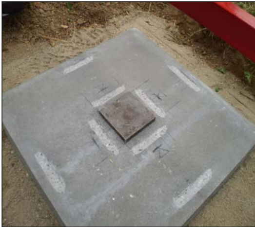
Fig. 3: Concrete tile prepared for tensionmetrical measurement, schema of tensionmeters location
