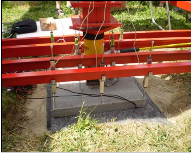
Fig. 2: Measuring of subsidence and concrete tile deformations
