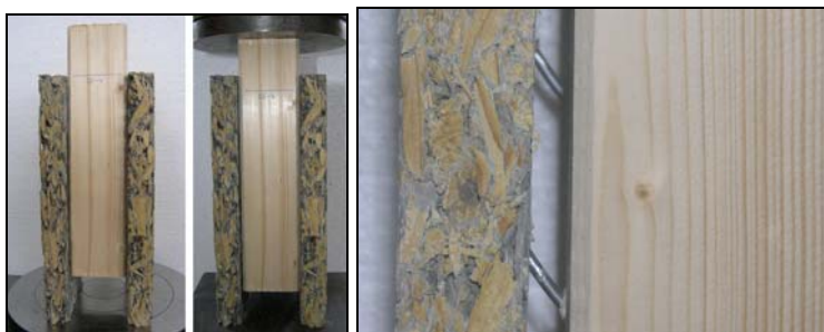
Fig. 6, 7: Test samples before and after destructive test procedure; typical damage of joint fasteners - nails
