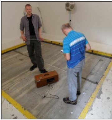
Fig. 6: Positioning of the source of impact noise
