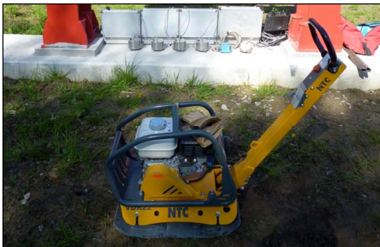
Fig. 2: VDR 22 reverse vibrating plate in experimental measurement
