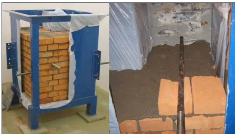
Fig. 1: Laboratory equipment and location prestressing bars in the masonry
