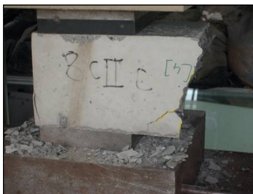
Fig.4: Test concrete beam 8C-IIC
