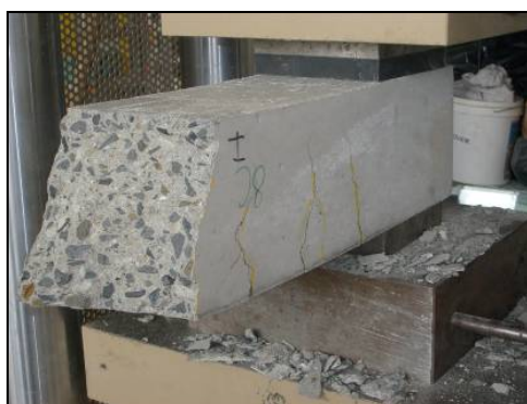
Fig.3: Test concrete beam 8C-IA (left) and 8C-IB (right)
