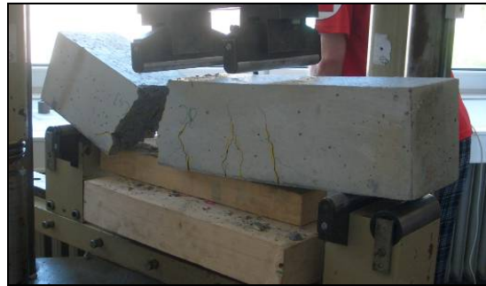
Fig. 1: Test beams after concrete work (left) and test beam, 8C – four-point bending (right)
