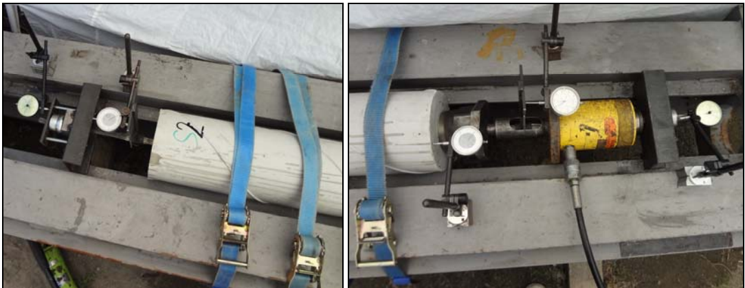
Fig. 3: Test arrangement, detail of passive and active side
