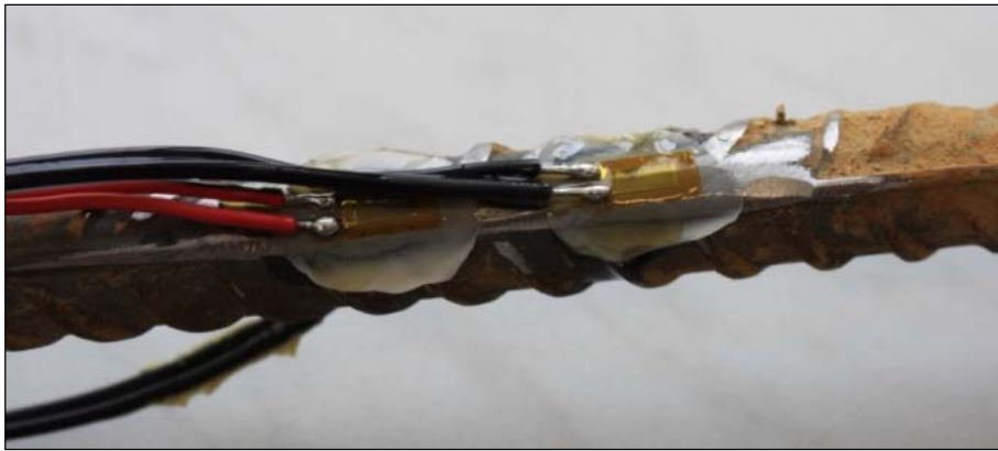
Fig. 2: Mounting of the foil one half bridge on the reinforcement
