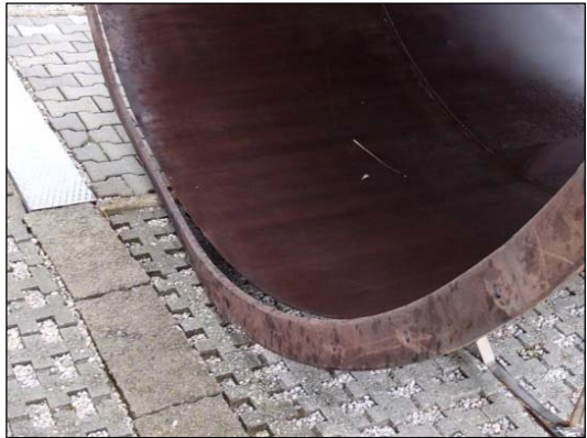
Fig. 12: Detached mount flange
