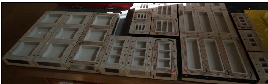
Fig. 10: Moulds designated for modCT specimens casting (accompanied with the three-point bending specimens moulds) (photo © Keršner 2013)
