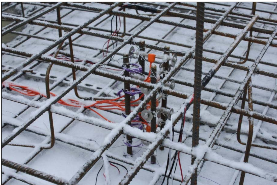
Fig. 1: Equipment for measuring the temperatures and strain in foundation slab
