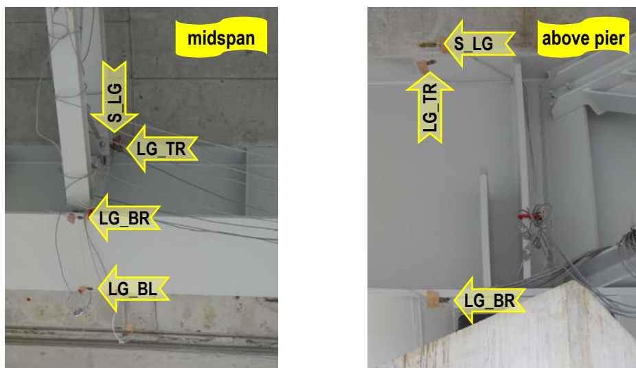
Fig. 3: Real position of several gauges in the "midspan" and "above-pier" cross-section
