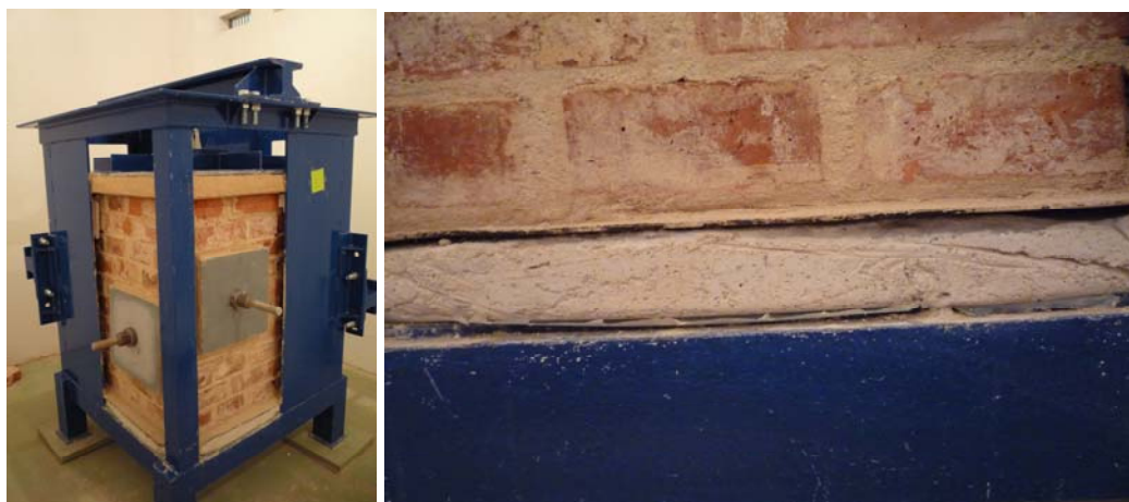
Fig. 2: Testing sample MAS_2, detail of sliding joint in the foot of masonry
