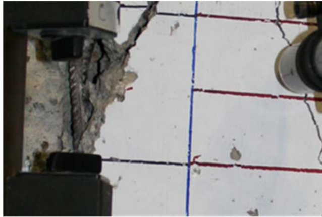
Fig. 19: Buckling of the longitudinal bar welds 4Ø8
