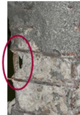
Fig. 11: Buckling of longitudinal bar of D_mRc-5_{\omega_c=0.15} after loading
