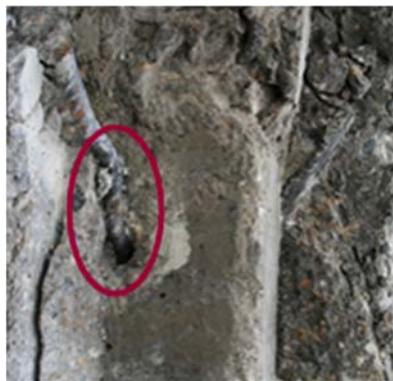
Fig. 20: Plastic region around the dowel bar - cut of specimen
