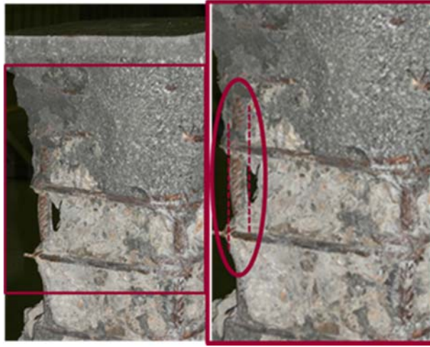
Fig. 7: Buckling of longitudinal bar of D_m R_c -5 \omega_c=0.15 after failure
