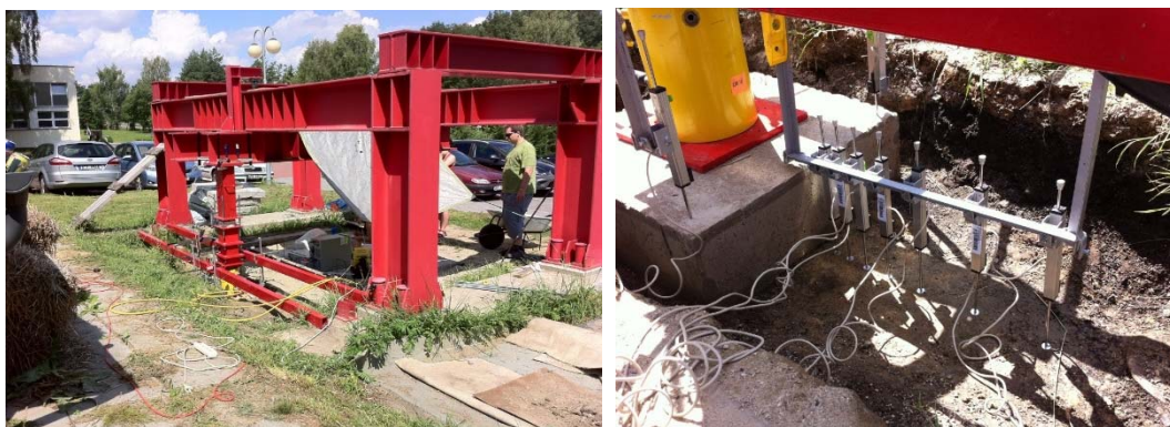
Fig. 5: Measurement on a model of the piled raft foundations (overview, a detail measurement of adjacent terrain)
