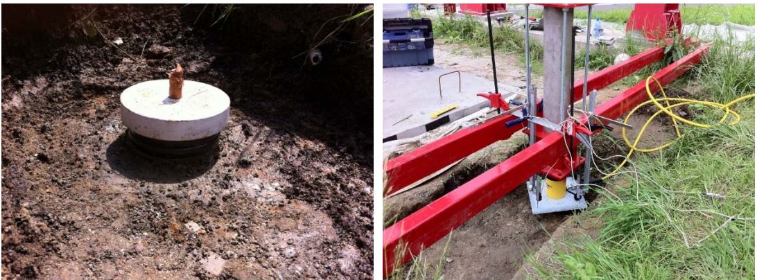
Figure 4: Measurement model of single pilot (with washers - left, measuring assembly - right)
