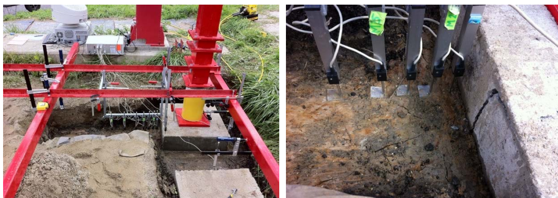
Figure 6: Measurement of model of slab (left – general view, right – the detail of terrain)
