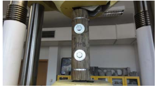
Fig. 7: Test – round wood # 11, humidity: 12 %, density: ca. 530 kg/m 3
