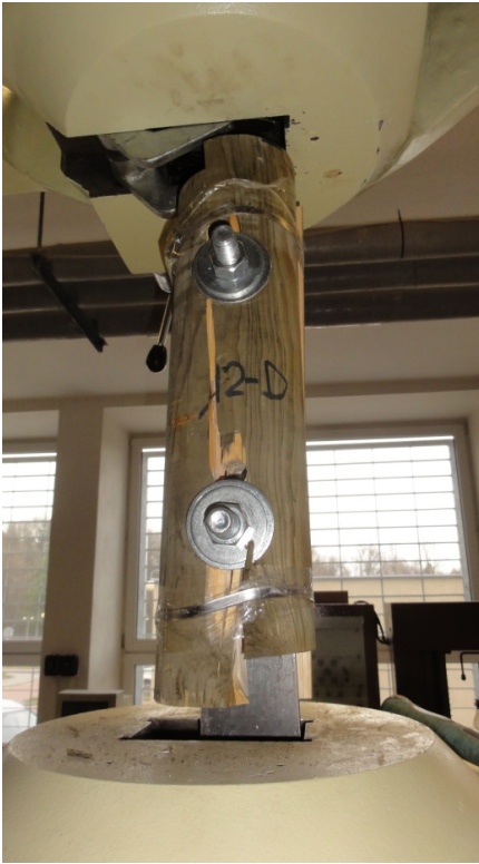
Fig. 21: The tested specimen reinforced with a band, and a numerical model with a bolt
