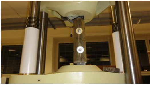
Fig. 6: Test – round wood # 9, humidity: 12 %, density: ca. 520 kg/m 3
