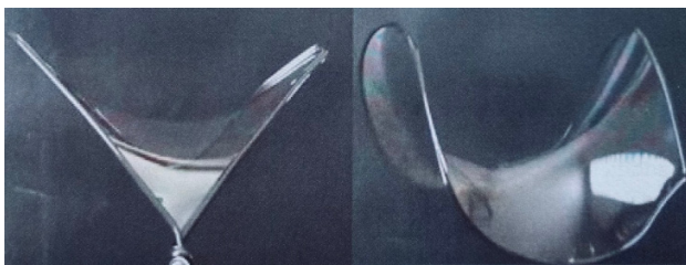
Fig. 3: Example of soap film model [2]
