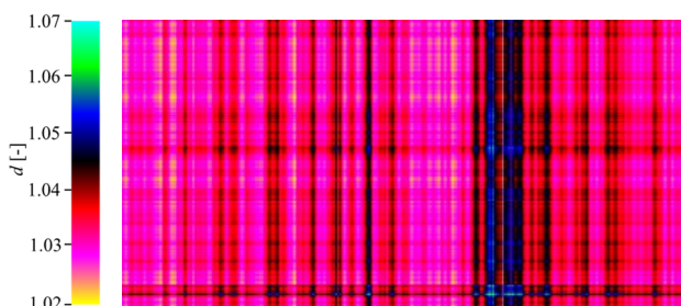
Fig. 9: Distribution of cross-dimension d_c measured on the whole surface.
