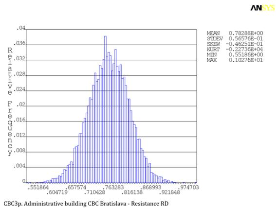
Fig. 8: Histogram of the resistance function  $RD = g(d)$
