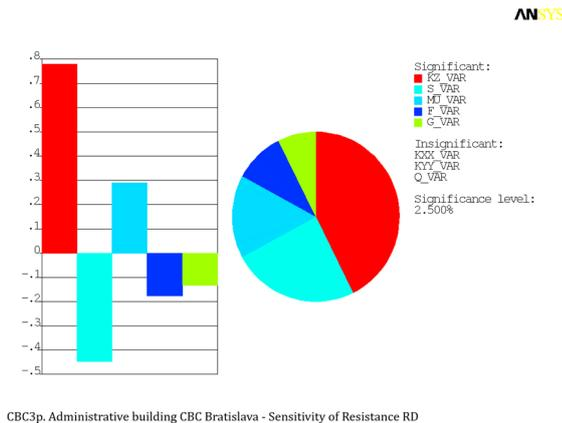
Fig. 6: Sensitivity analysis of the resistance function  $RD = g(d)$
