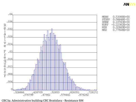
Fig. 9: Histogram of the resistance function  $RM = g(M)$
