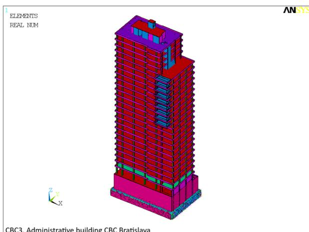
Fig. 3: Calculation model CBC3 with 3D soil model.
