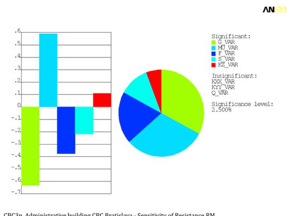
Fig. 7: Sensitivity analysis of the resistance function  $RM = g(M)$
