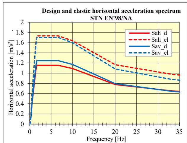
**Fig. 4:** Acceleration spectrum according to STN EN 1998/NA
