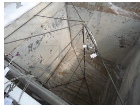
Fig. 4: Layout of the sensors on the top of mock-ups.
